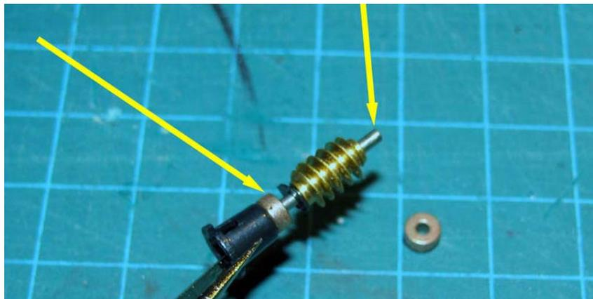
Don't re-install the worm yet – we will lubricate the drive axles and gears before completely reassembling the gearbox.
