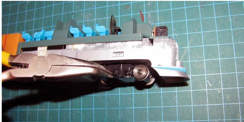
The final step is to reinstall the nose. Start by placing the bottom tabs on their seats in the shell, and then snapping the top into place.
