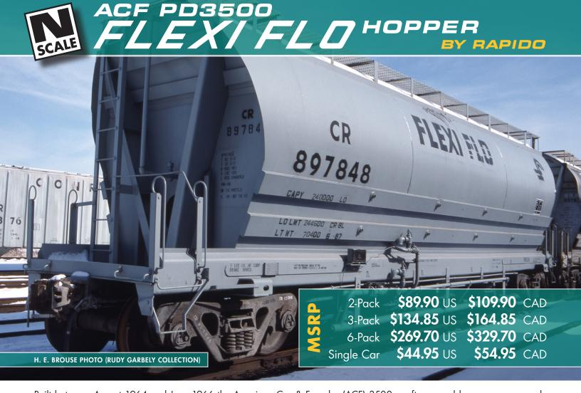
Built between August 1964 and June 1966 the American Car & Foundry (ACF) 3500 cu. ft. covered hopper was an early innovator in pressure differential unloading and a marketing masterclass thanks to the **"Flexi Flo"** tag coined by the car's biggest customer, the New York Central railroad.
